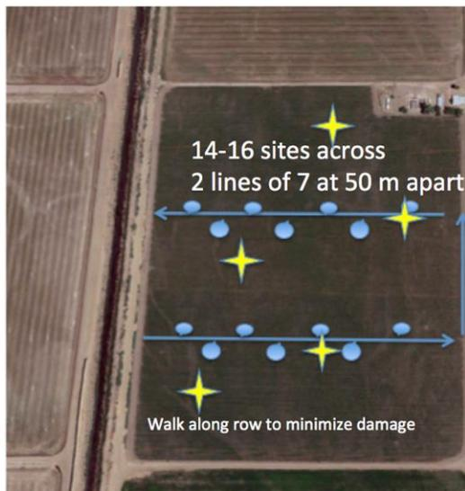
Fig. 8.1.1.1. Example layout of instrumented stations (yellow star) and temporary intensive manual locations (blue circle) for *in situ* soil moisture reading at a super site for post-launch validation.
